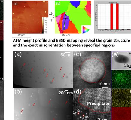
S/TEM analysis of PbSe-10%Cd. Decent amount of triangular shape CdSe precipitates are observed, super-structured interface appears to compensate the lattice misfit
