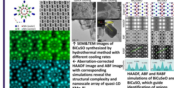
↑ SEM&TEM images of BiCuSO synthesized by hydrothermal method with different cooling rates
