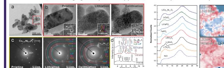
In-Situ TEM studies observe lithiation and delithiation of Cu<sub>2</sub>Ni<sub>1-x</sub>F<sub>2</sub> to understand sources of capacity fade
